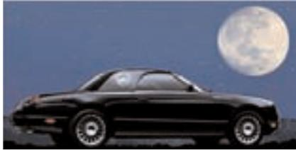
Many car models now use this technology; for example, Ford's Thunderbird has plastic bumpers, hood and bonnet, and most UK cars today have a much higher proportion of plastics which have replaced metals. An additional advantage of plastic components is that they are cheaper to produce, in different colours, than metals, which require a smooth surface before they are painted with several coats.
