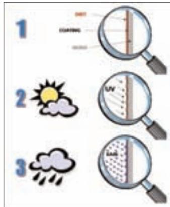
On a building like an all-glass skyscraper, new windows with this coating are a real bonus since they do not need cleaning as much as normal glass, and window cleaners in cradles do not have to operate so often.
