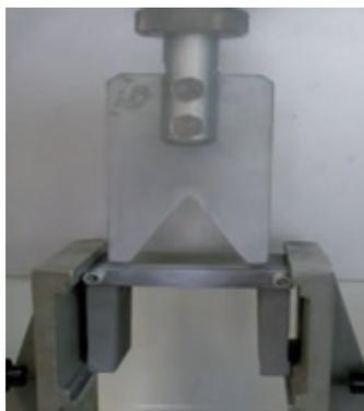
Figure 2: Varner-Bratzler shear probe.
