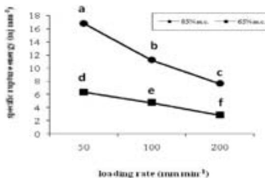
Figure 8: interaction effect of moisture content and loading rate on specific rupture energy.
