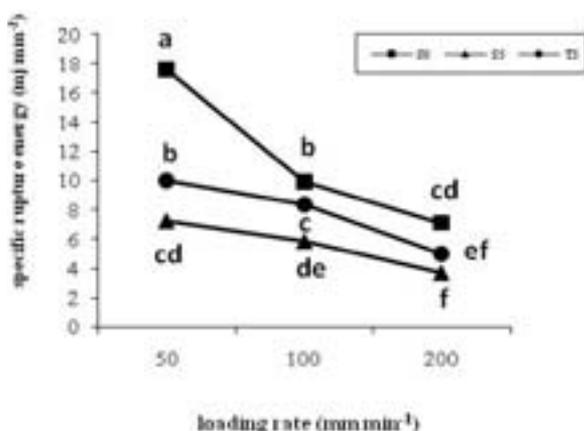
Figure 6: interaction effect of loading rate and loading type on specific rupture energy.
