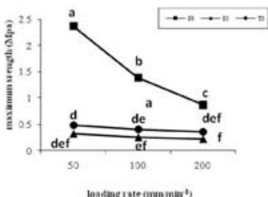
Figure 5: interaction effect of loading rate and loading type on maximum onion leaf strength.
