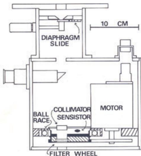
Figure 7a. The RFC photometer.
