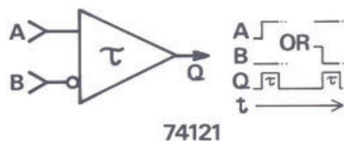
Figure 2. Operation of mono stable oscillator.
