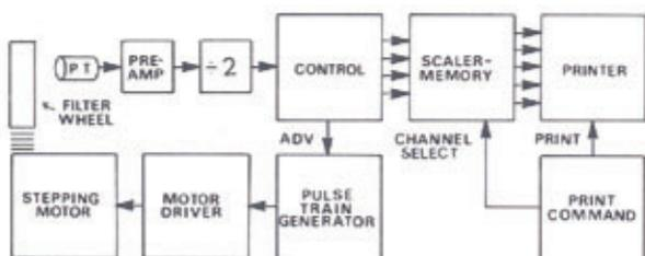
Figure 1. Block diagram of the photometer electronics.
