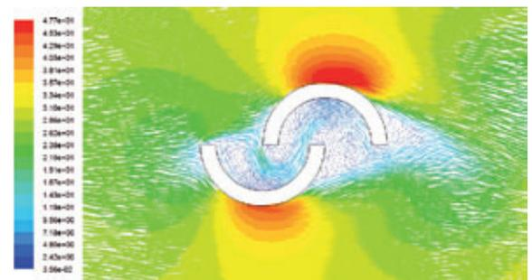
Figure 10. Velocity contour for 25% overlap.
