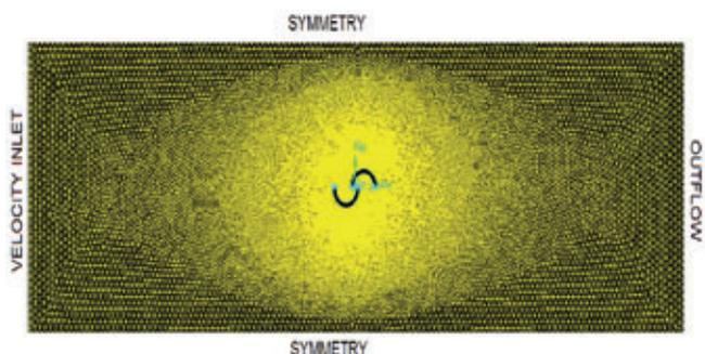
Figure 3. Physical model, boundary conditions and computational domain of the Savonius rotor at 16.2 overlap condition.
