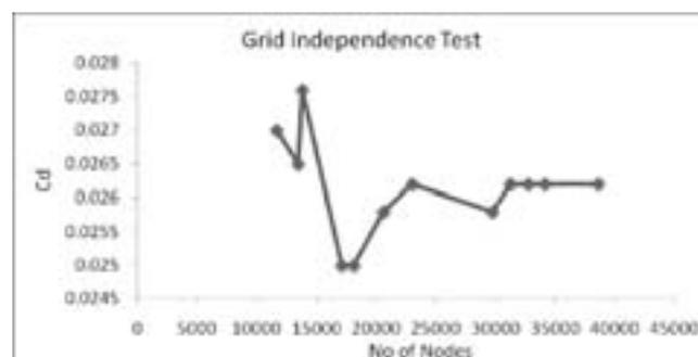
Figure 4. Grid independence test carried out for a two-bucket S rotor.
