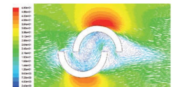
Figure 14. Velocity contour for 35% overlap.
