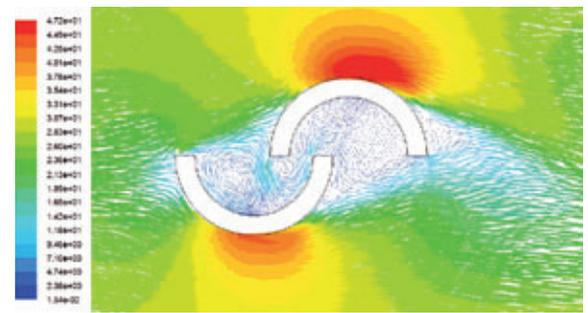
Figure 8. Velocity contour for 20% overlap.
