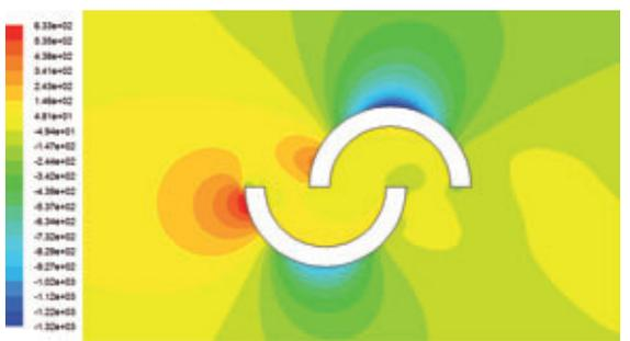
Figure 11. Pressure contour for 30% overlap.
