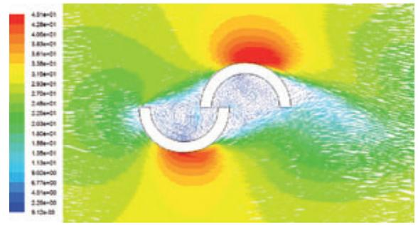
Figure 6. Velocity contour for 16.2% overlap.
