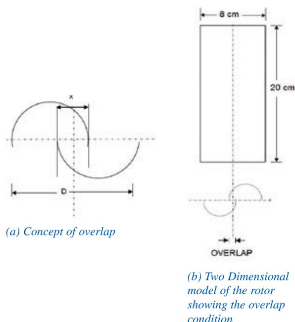
Figure 2. A Savonius Rotor showing the overlap condition.
