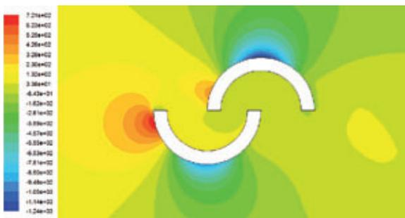
Figure 9. Pressure contour for 25% overlap.
