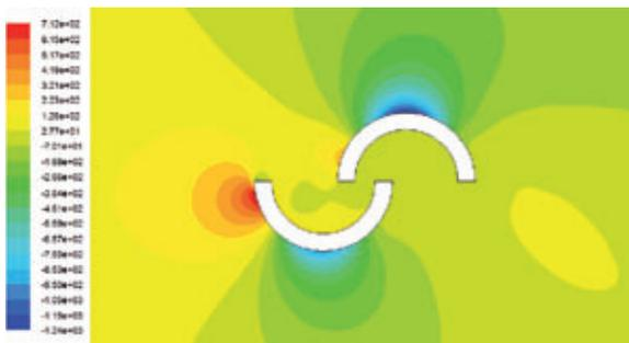
Figure 7. Pressure contour for 20% overlap.
