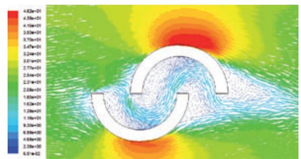
Figure 12. Velocity contour for 30% overlap.
