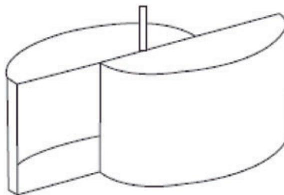
Figure 1. A two-bucket Savonius rotor showing overlap condition.
