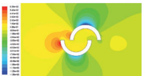
Figure 13. Pressure contour for 35% overlap.
